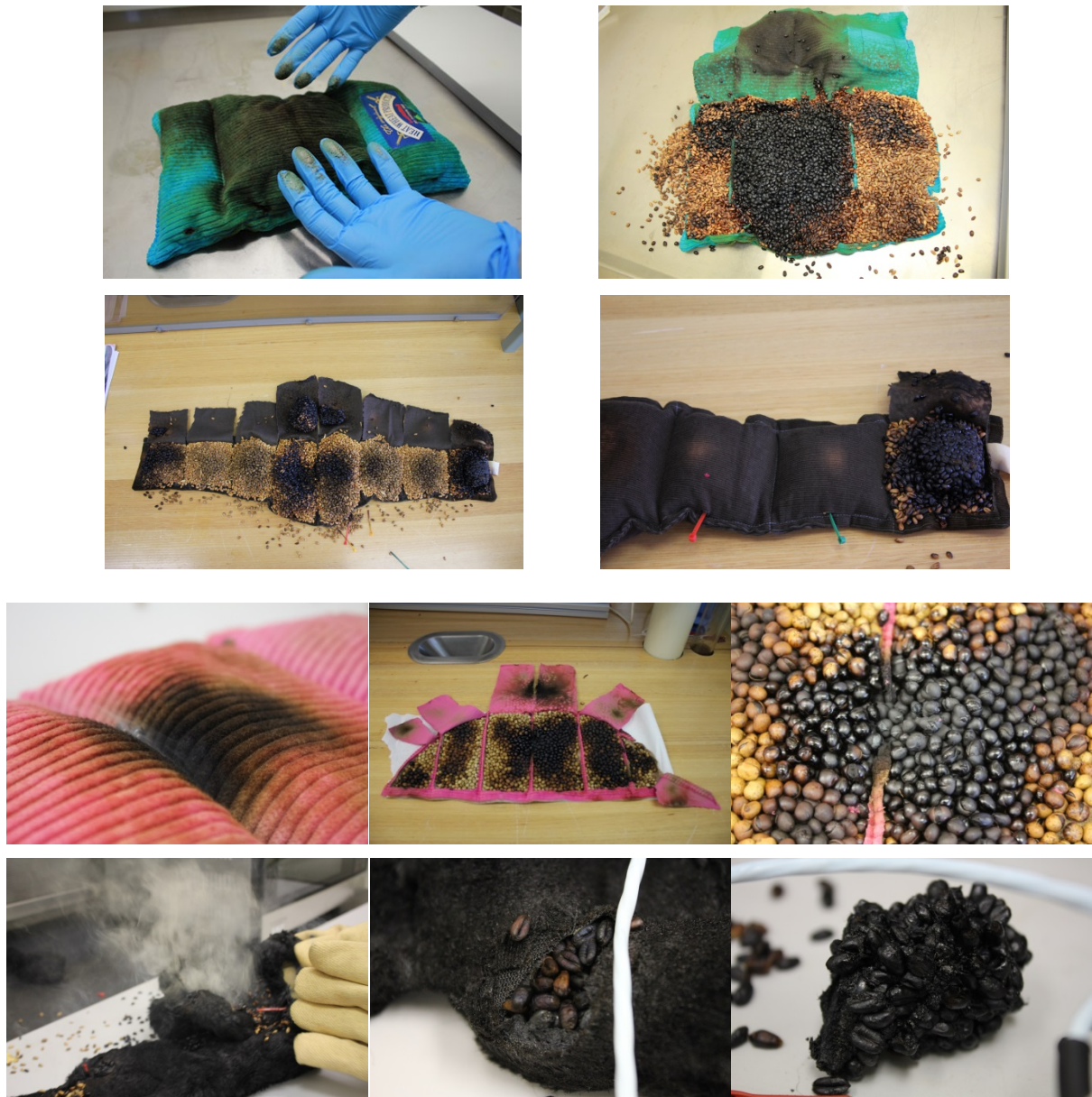
Figure 4: Charring of heat pack filling material.
