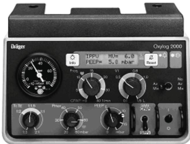
Investigation of the ventilator and circuit found that a valve had been placed upside down in the circuit. The valve had been put in the wrong way during cleaning and reassembly and was not detected until the users began troubleshooting when the ventilator continued an alarm. The issue was further compounded by procedural errors and the ventilator issuing two alarms at the same time.
