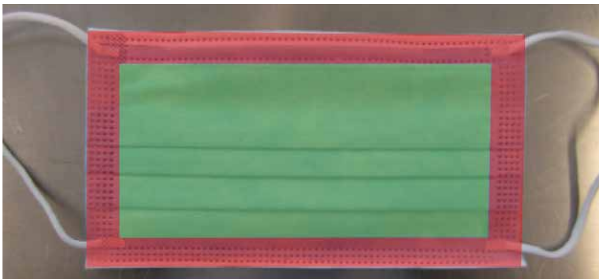
Figure 2 – Main body (green) of the surgical/medical facemask must be tested for fluid resistance; the perimeter region (red) can be excluded from the testing.
