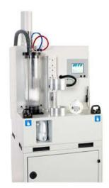
Penetration, filter resistance and flow rate data are transferred in near real time via USB cable to a nearby connected laptop running data acquisition program recording values and producing charted plots of resistance and penetration.
